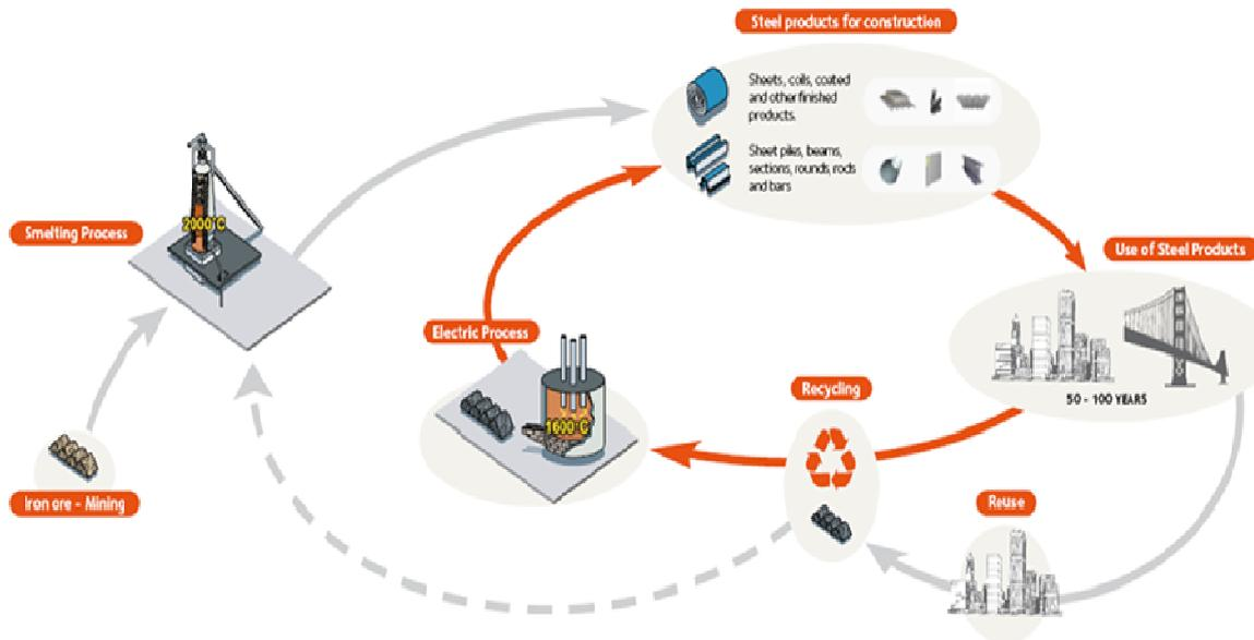
Figure 1-2 : The steel recycling loop
